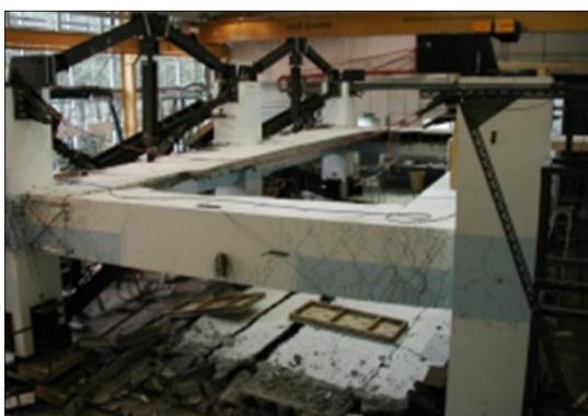
(a) Unit failure during “system” test (Mathews, 2004)
