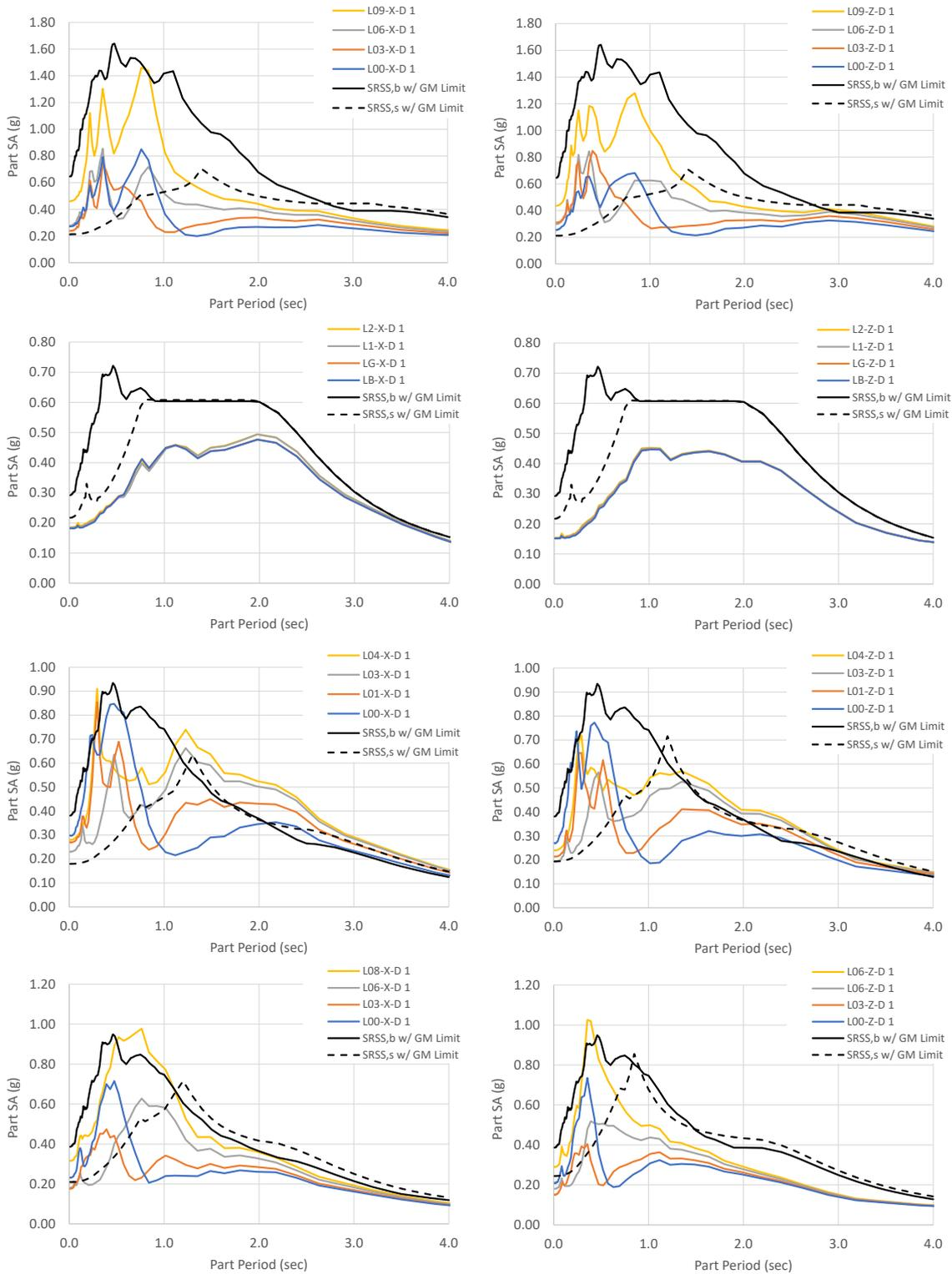
Figure 7. Processed floor acceleration spectra from NLTHA recorded acceleration traces at the diaphragm centre-of-mass including prediction using the Welch & Sullivan method (2017) (a) Building 1 (b) Building 2 (c) Building 3 (d) Building 4. Solid black curve represents  $m_b$  response, and dashed black curve  $m$  response.
