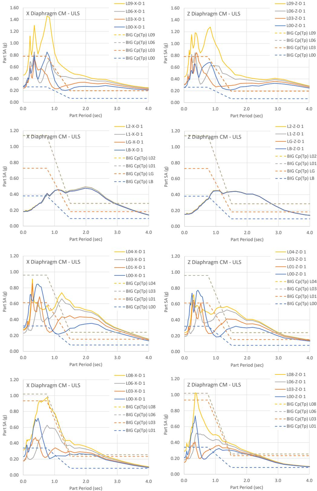
Figure 5. Processed floor acceleration spectra from NLTHA recorded acceleration traces at the diaphragm centre-of-mass, including predicted spectra following the NZSEE seismic isolation guideline (a) Building 1 (b) Building 2 (c) Building 3 (d) Building 4.
