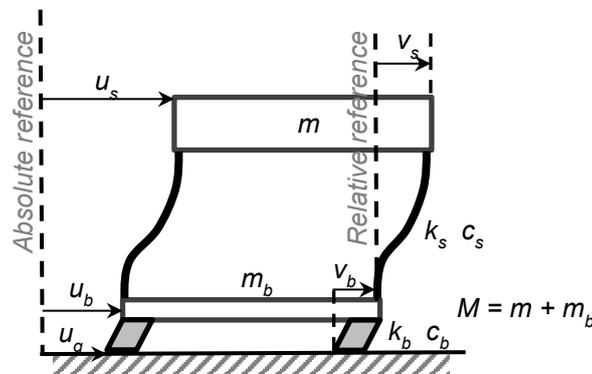
Figure 6. Two-degree-of-freedom representation of superstructure + isolation response
