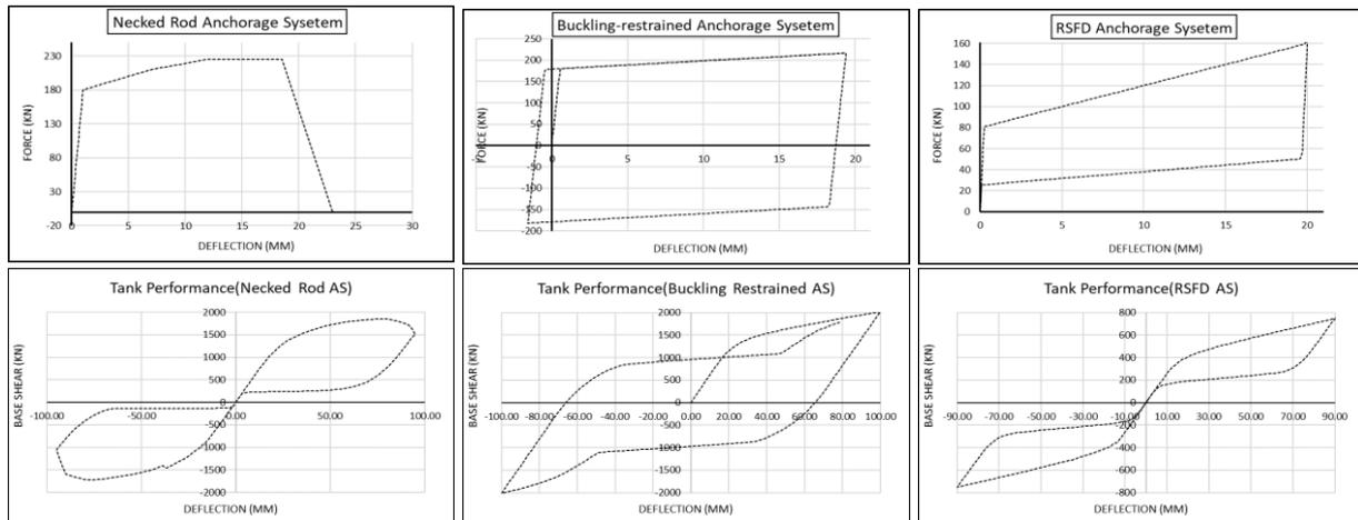
Figure. 6 – The hysteresis behaviour of joints and tanks for three introduced mechanism
