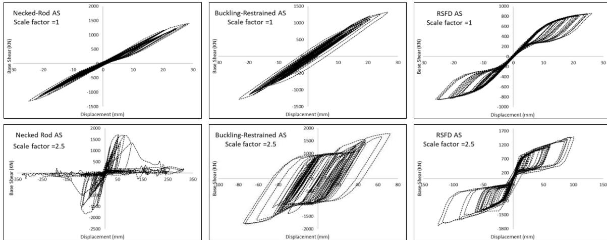
Figure. 10 – Tank hysteresis for the investigated anchorage systems subjected to Kobe record
