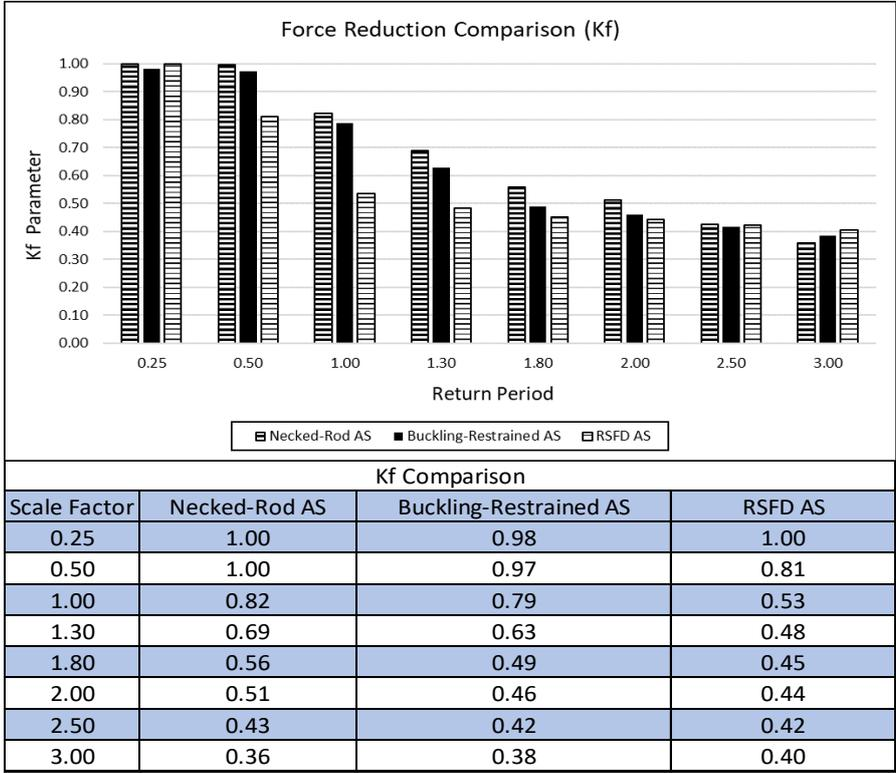
Figure. 9:  $k_f$  values for different amounts of the return period
