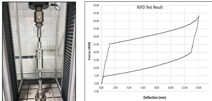
Figure. 2 – RSFD test setup and performance test result [11]
