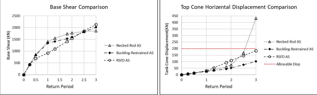
Figure. 8 – Base shears and top tank’s cone displacements subjected to seven selected records
