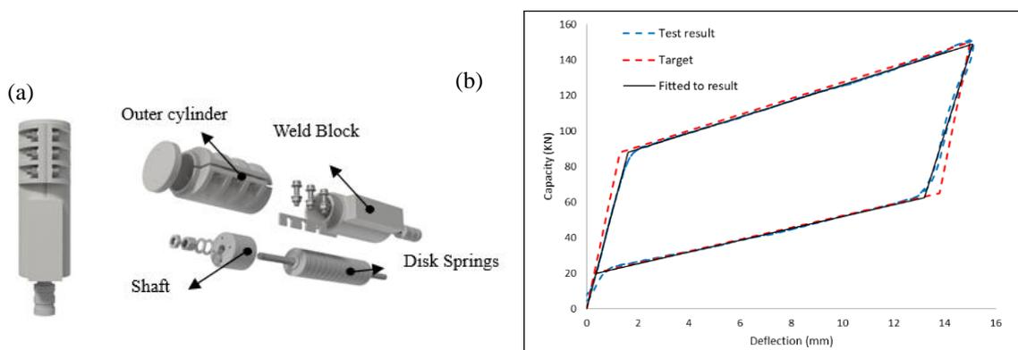
Figure. 3 – (a) RSFD components (Left); (b) Test result (Right)
