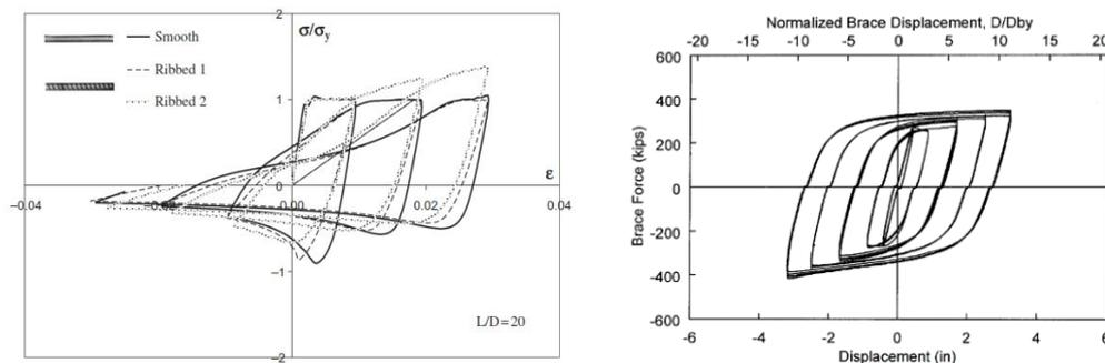
Figure. 4 – (a) Hysteresis performance of the necked rod [12] (Left); (b) Buckling-restrained behaviour [13] (Right)
