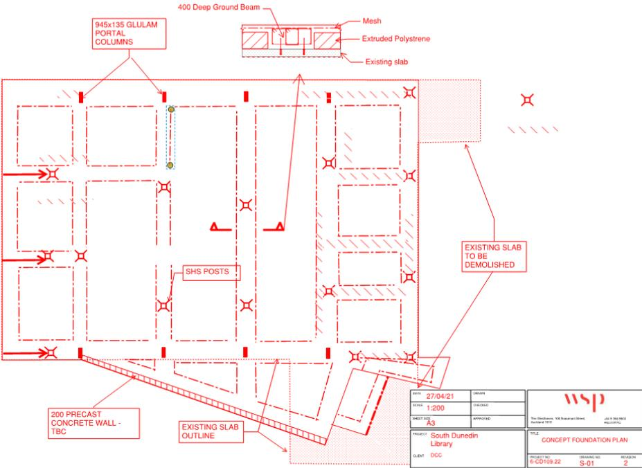
Figure 4. Concept foundation plan
