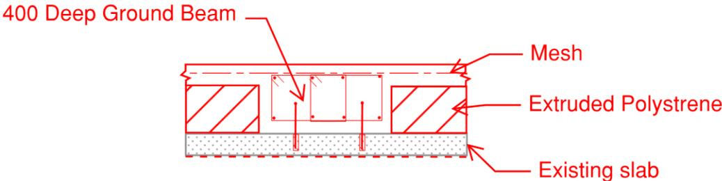
Figure 6. Preliminary typical foundation detail
