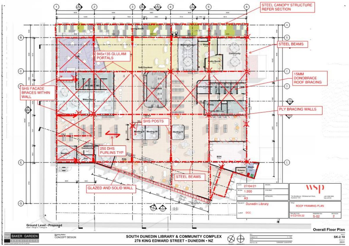
Figure 3. Concept roof framing
