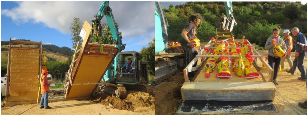
Photographs 1 and 2 – Full scale out of plane tests of low density adobe walls
