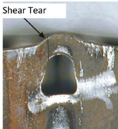
Figure 4: A downstream bolt failure in shear tearout (Cai and Driver, 2010)
