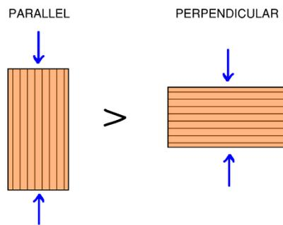
Figure 6. Timber is much stronger parallel to the grain than perpendicular
