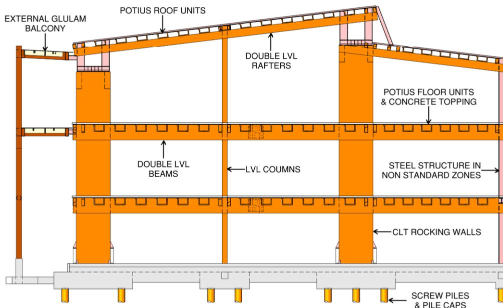
Figure 2. Typical Building 1 cross section
