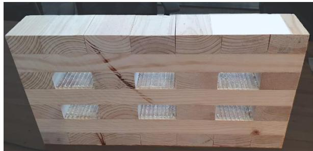
Figure 5. CLT duct sample
