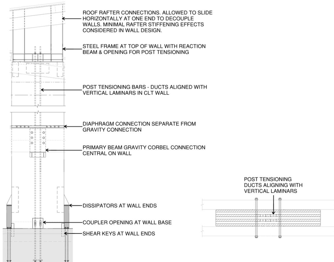
Figure 3. Key features of a typical CLT wall
