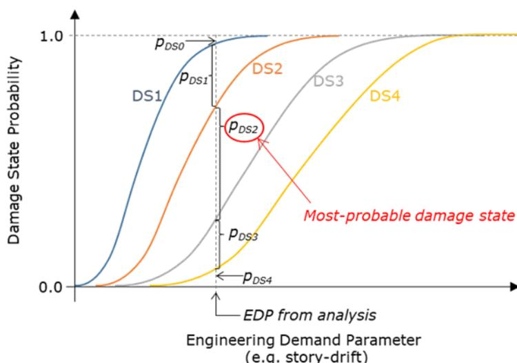
Figure 3: Use of fragility curves to identify probable damage state.
